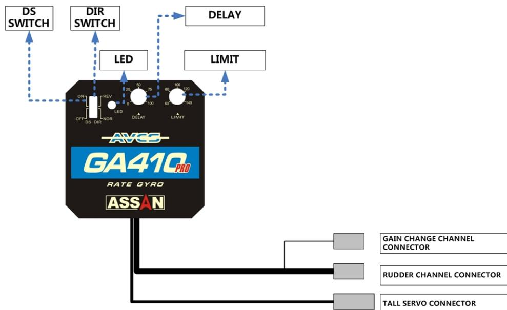
1. DS SWITCH: The ON position is for high speed signal Digital servo only
