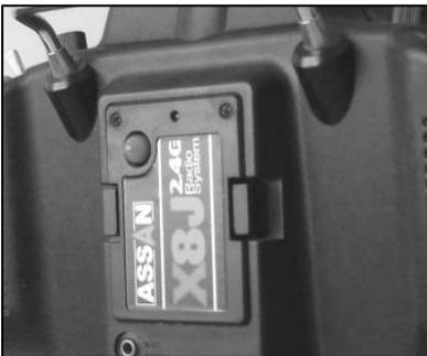
Take the ASSAN X8 2.4GHz transmission module that matches the transmitter out of the package. Don't fix the antenna for now and be careful not to damage the exposed screw thread part of the antenna pedestal.
