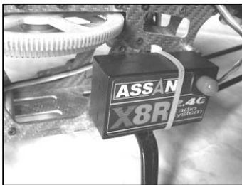
When the installation position is determined, fix or bind the receiver onto that position. Do not use the metal or metal-involved materials or any conducting material as the fixture or binding material.
