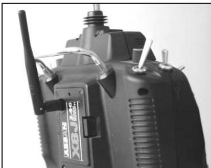
Unscrew the red plastic protective cap off the antenna pedestal (counter-clockwise). Insert the plug of the 2.4GHz antenna right into the antenna pedestal and screw the coupling nut of the antenna clockwise
