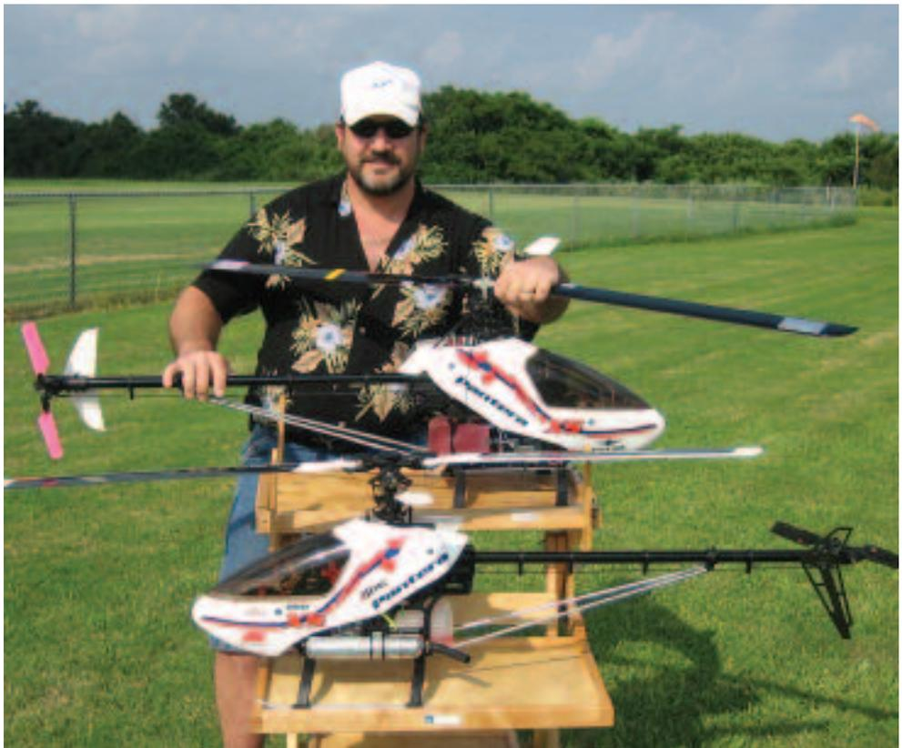
Fellow club member James Lerch with two Pantera 50s on steroids. His YS 80-powered machine was clocked at 89mph, while mine has a YS 60 with Mavrikk 620 rotor blades to handle the extra power. We both use JR7100R receivers with RevLimit to keep the engines within operational limits. This excessive performance isn't required for normal flying, but it's great to have when needed.
